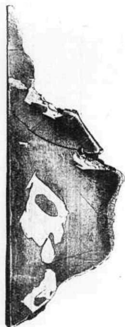
Fig. 3.—Etched surface of the La Primitiva Meteoric Iron showing Schreibersite. (Natural size.)
