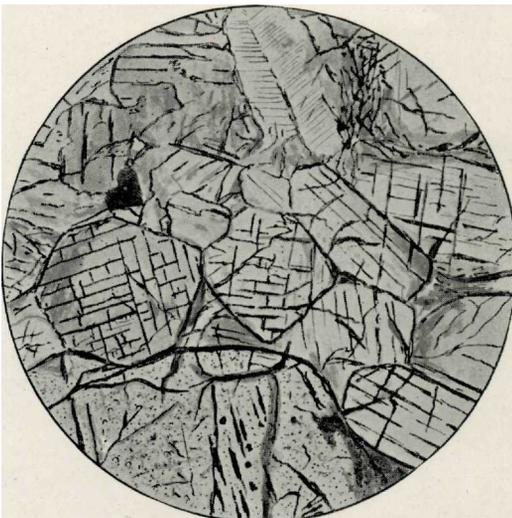
FIG. 3. Thin section of meteorite, magnified 20 diameters. The upper three-fourths of the figure show augite-crystals in basal and prismatic section. At the top of the field, a twinned augite-crystal showing herring-bone structure. At the bottom of the figure, part of a large crystal of hypersthene, containing opaque inclusions.
